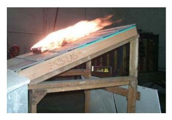
Combustible roofing materials, to include wood, fiberglass, etc. are subject to ignition from fire embers and brands. Many homes that ignite in wildland urban interface fires burn from the top down; this is a result of ignition of the roofing materials or the combustible roof decking.
